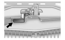
Go to the front of the vehicle and find the secondary hood release lever. The lever is located under the front edge of the grille near the center. Push the release lever up and raise the hood. Before closing the hood, be sure all the filler caps are on properly. Then pull the hood down and close it firmly.
